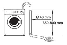
The hose must not be sticked into the standpipe more than 50 mm and it has to be fixed in this position. The drain hose must not be kinked.
